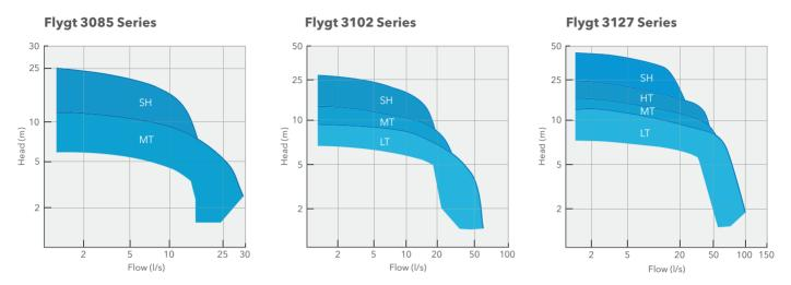
Pressure Characteristics: SH - Super High Pressure, HT - High Pressure, MT - Medium Pressure, LT - Low Pressure
