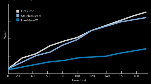
After 200 hours, the Hard-Iron impeller proved to be five times more wear resistant than the grey iron version. The stainless steel impeller showed wear comparable to the standard grey iron material.
