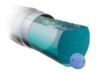
The SmartBall® platform is a free-swimming inspection tool used to detect leaks and gas pockets and map pipeline networks. This platform assesses pressurized water and wastewater pipelines in a single deployment, without disrupting regular service. The SmartBall platform provides utilities with pipeline condition data to make informed rehabilitation and management decisions on a pipe-by-pipe basis.
