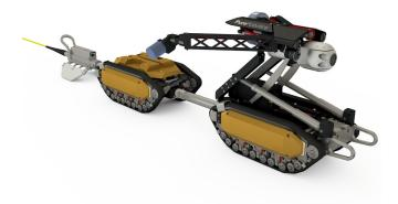
The PureRobotics® platform is a modular, multi-sensor condition assessment tool for depressurized water pipelines. Using accurate electromagnetic and other sensor data paired with live video, this platform provides utility owners with comprehensive pipe wall condition data used to make rehabilitation and management decisions on a pipe-by-pipe basis.
