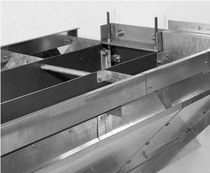
Leopold Trough-Guard media baffles are constructed of corrosion-resistant Type 304 Schedule 5 stainless steel and can be bolted onto concrete, steel, or FRP troughs.
