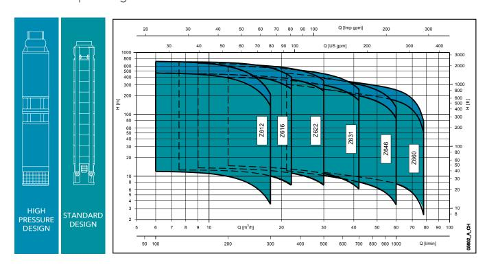
Z6 series operating characteristics at 60 hz.
